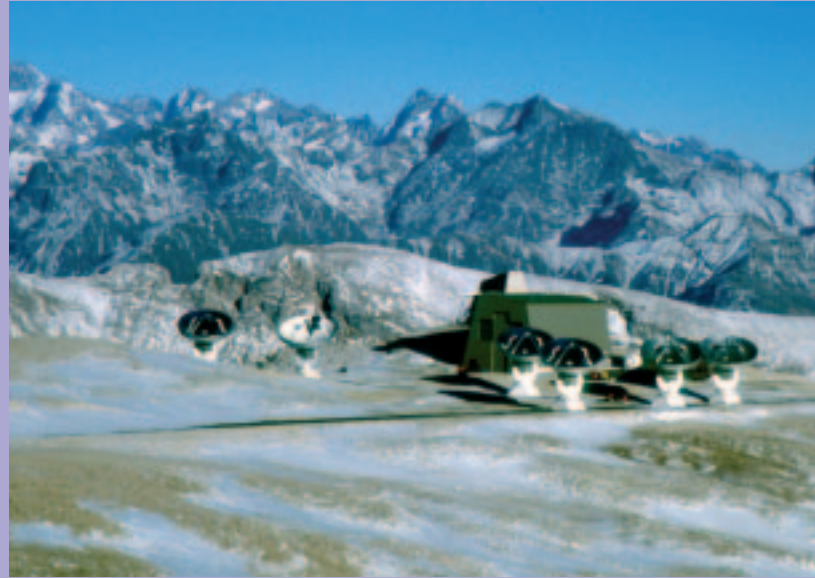
The IRAM Interferometer in the French Alps combines six antennas to obtain a higher angular resolving power
